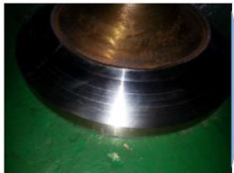
< Inconel625/718 welded Spindle disc >
