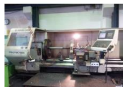
< Machining welded part of disc making groove for inconel718 >
