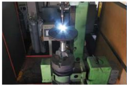
< Inconel625 welding on bottom & side surface >
