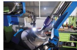
< Inconel 718 welding on spindle disc >
