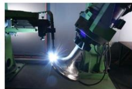
< Inconel625 welding on spindle disc >
