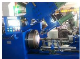
< Rolling on Spindle disc >
